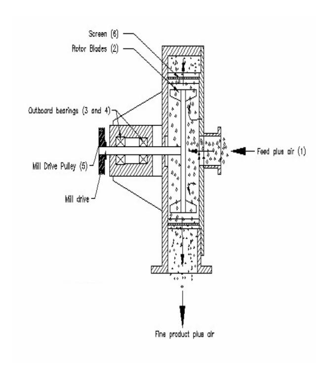
Figure 6.8: Operating Principle
