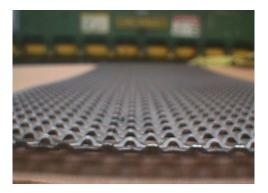
The picture at the left shows a view looking down the forward direction of the screen. In this direction, the hole openings are visible to the eye. When these holes face the direction of rotation of the grinder rotor, the screen is installed in the "forward" direction. In this manner, proper air and product flow is maintained.
