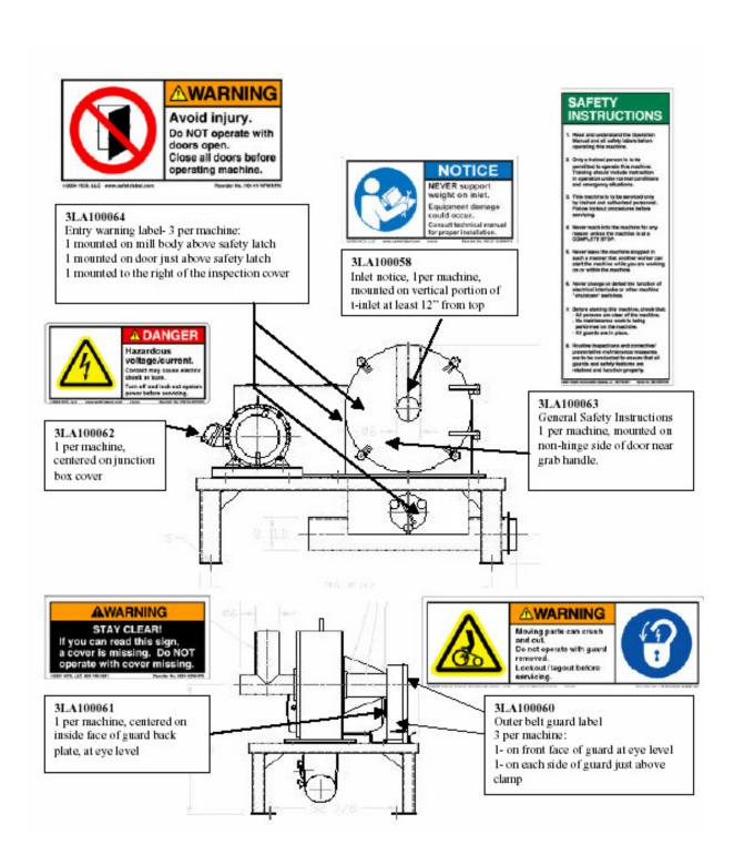
Illustration 1-3: Fine Grinder Safety Label Placement for standard and explosion proof mills
