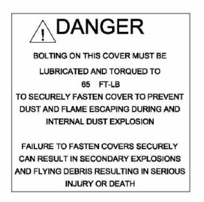
Illustration 1-4: Fine Grinder Safety Label Placement for standard and explosion proof mills
