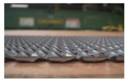
The picture at the left shows a side profile view of the screen. As you can see, the stamping process for this screen creates a form very similar to a cheese grater. These screens would be installed in the forward direction when the direction of rotation of the grinding rotor sweeps left (relative to the picture shown).
