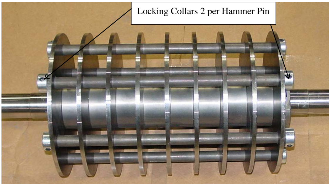
Figure 5-8: Detail of Locking Collars
