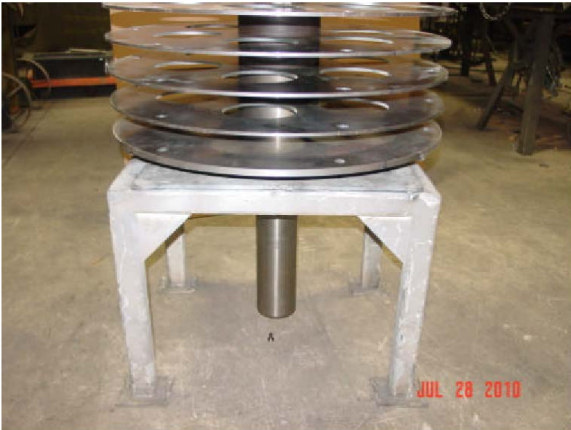
Figure 5-16: Rotor in stand for disassembly and reassembly
