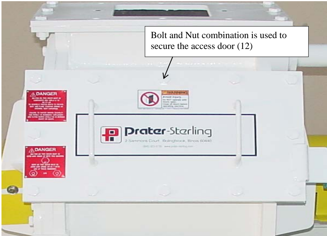
Figure 5-6: G PSR 11 Hammer Inspection/Removal Access Door
