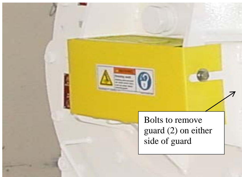
Figure 5-12: Non-Drive Side Bearing/Shaft Guard
