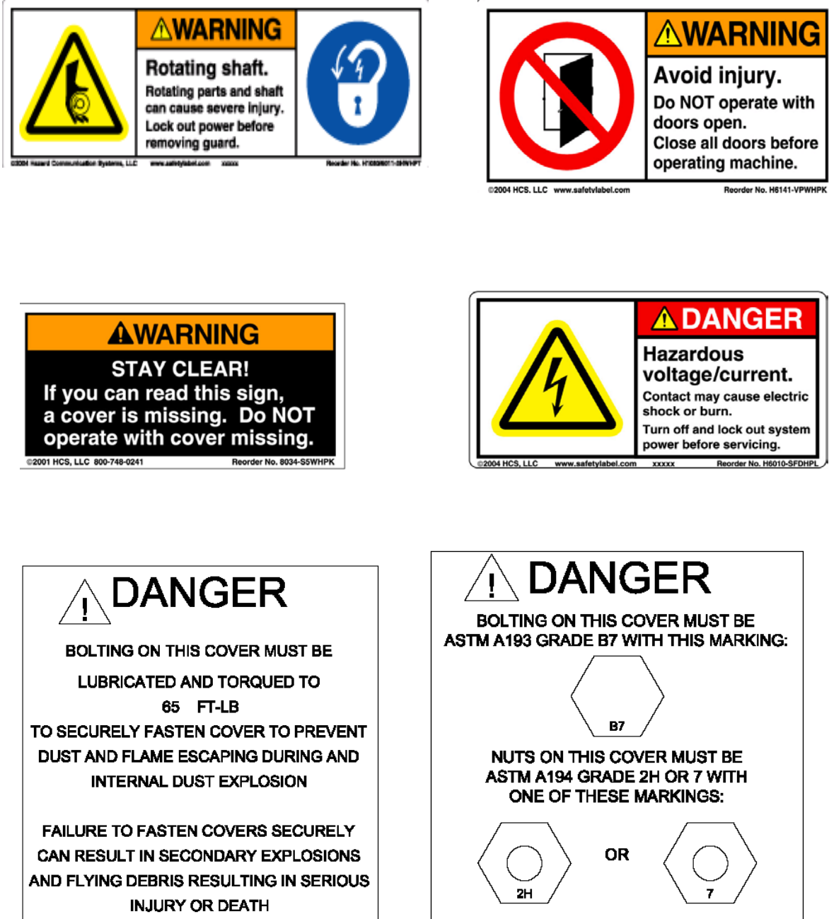
Figure 1-2: Safety Labels for the G PSR 11 Series
